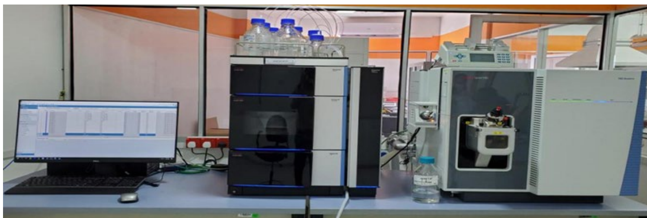
LC-MS/MS Instrument at SGS Lanka Pesticide Residue Laboratory
